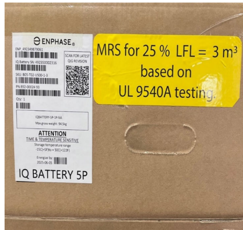
Figure 4: Packaging label showing Enphase unit part number and minimum room size
